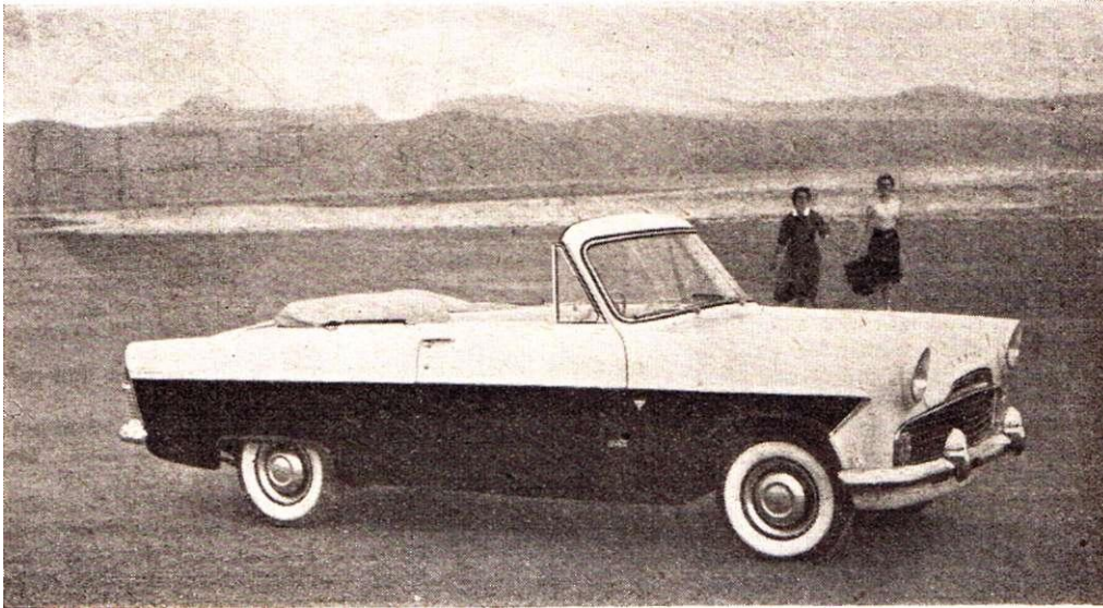
DISAPPEARING side windows are a feature of the new Zodiac convertible, but when the power-operated top is raised large quarter lights give safe and convenient all-round vision from the driving seat.
