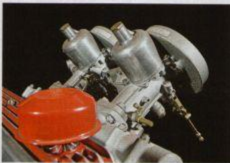
Raymond Mays two-carburettor conversion transformed 85mph Zephyr workhorse into a 100mph stallion
